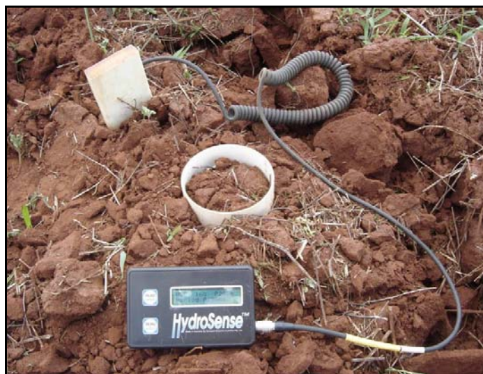
Fig. 03 – Hydrosense system (TDR).
